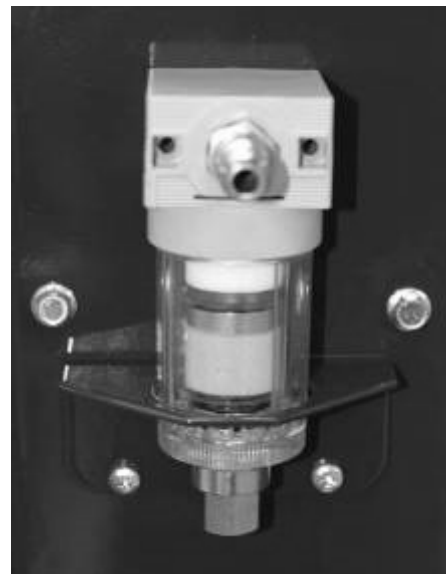
Air connector Screw the air connector on the back of the air filter.
