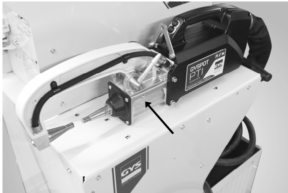
Assemble the clamp handle on the left side of the clamp
