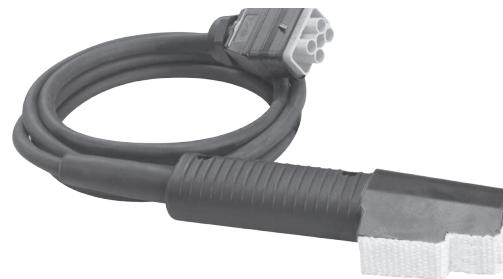
The bolt inductor is used for intense heating of rusted or stuck parts such as nuts and bolts. When using the Bolt inductor to loosen stuck nuts and bolts, it is OK to use full power to start with. Other uses include caulking removal from truck beds and trunks of sedans, as well as soldering large electrical connectors and metal forming.
